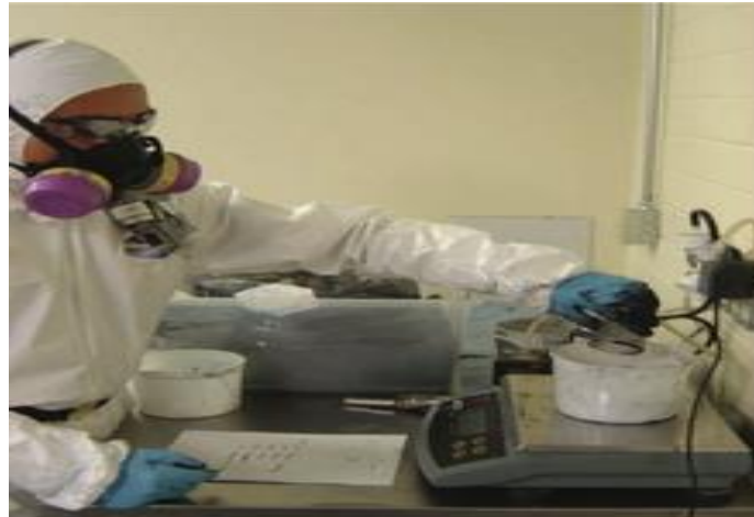
Figure 4: A worker wearing a respirator, lab coat, and gloves while weighing carbon nanotubes
