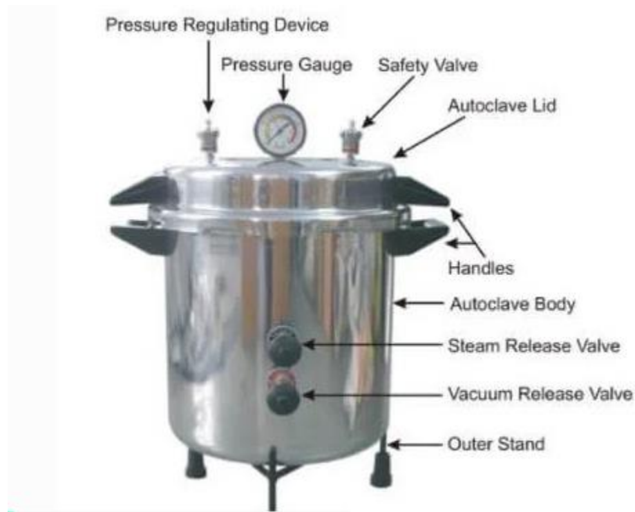
Figure: Autoclave Parts or Components. Image Source: pharmawiki .
